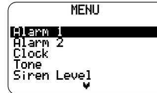
2. Choose Time and press the SELECT button, and the hour setting will begin flashing. Use the TUNE UP/DOWN to set the hour as desired. Note: the AM/PM setting is affected by the hours setting. Press the VOL UP to the minutes setting. The minutes will begin flashing. Use the TUNE UP/DOWN to set the minutes as desired.
