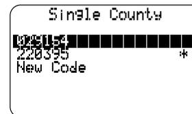
3. Under Multiple County mode, repeat the same instruction as above to set up, edit or enable / disable your FIPS codes. To leave the current operation, press the MENU button once.
