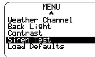
2. Press the TUNE UP/DOWN to test the siren. The radio will sound a sample of the siren of each warning level.
