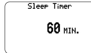
2. Continue holding the STANDBY button and the Sleep Timer will automatically start switching between the 6 settings. Release the STANDBY button when the setting switches to the time desired to set as the preset sleep time. The sleeper icon "
