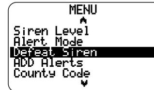
2. Press the SELECT button to enter the Defeat Siren menu. The words ADMINISTRATIVE MESSAGE will scroll across the bottom of the LCD display. This is the first alert on the list of alerts that NOAA can broadcast. You have the option to disable the siren to block this alert or enable to receive it. Use the VOL UP/DOWN to make your selection.
