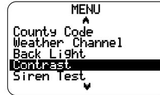
2. Press the SELECT button to enter the Contrast menu. Press the VOL UP/DOWN to adjust the Contrast level. Press the SELECT button to save the setting. Press the MENU button to exit to main menu list.
