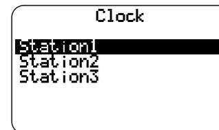
3. Select Station1, Station2 or Station3 to set up the radio frequency (FM) as the source station of the radio CT. The radio will synchronize the clock time according to your settings of these three stations every two hours. The
