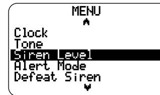
2. Press the SELECT button to enter the Siren Level menu, then press the VOL DOWN/UP to select the desired volume setting between Low, Middle and High. With each setting the radio will sound a sample of the appropriate siren volume.
