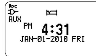
3. Your radio will switch off after the preset time has elapsed. To cancel sleep timer, simply press the STANDBY button to turn off your radio.
