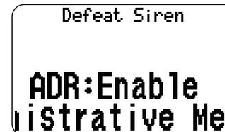
3. After setting the Defeat Siren for this alert, use the TUNE UP/DOWN to scroll through the list of alerts, following the same sequence to set the Siren Mode for each alert desired.
